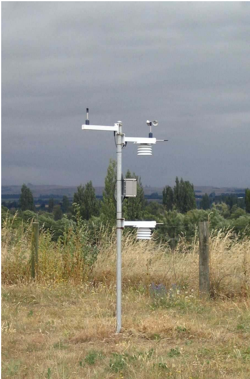
Figure 2 Weather station configuration: Screened (air temperature) and exposed temperature sensors at the standard meteorological height of 1.2 m, and at 0.9m above the canopy (ie at 2m). Wind speed and direction (vane in line with view) are also measured at approximately 2m.
