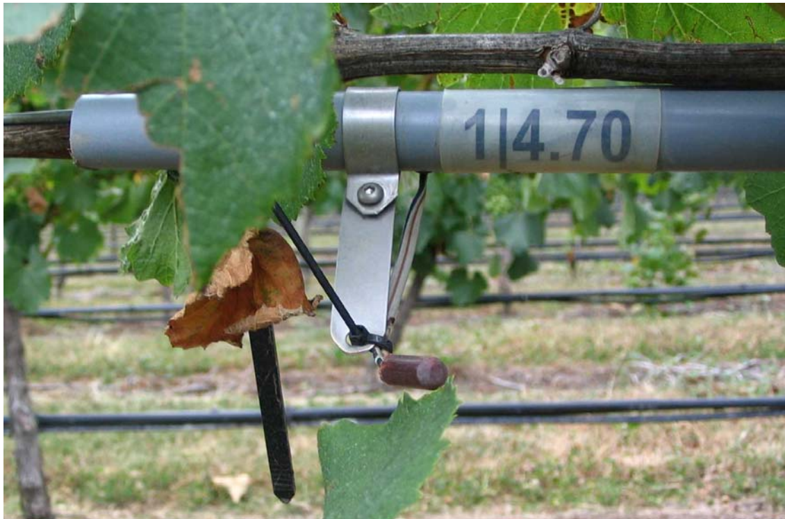
Figure 3 In-vineyard bud temperature sensor with label referring to sensor number and distance from data logger (and hence sprinkler) of 4.7m.
